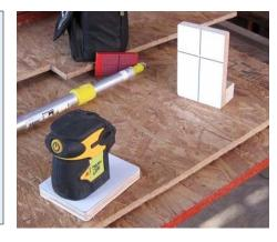
Truing up walls can be especially tricky using even a plate to plate level. This makes using a laser plumb bob a lot easier. The 2" offset from the front and sides allows the unit to be placed in a corner and both walls trued up. And the target can easily be seen by several people making truing up walls a task for a 'team'. The red target reflects the laser dot and makes this very usable in even bright sunshine.
