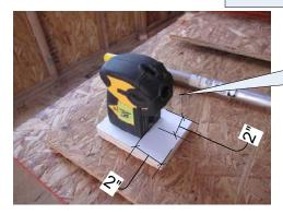
Laser Plumb bob attached to a piece of particle board with a short machine screw into bottom tripod mount.
